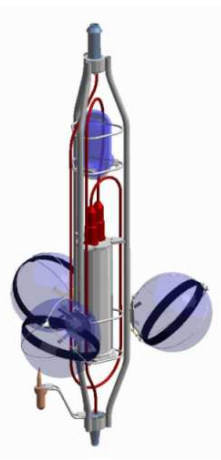
Figure 2. An artist’s view of the ANTARES detector (left, not to scale) and a schematic view of a storey (right) with the three glass spheres for the photomultipliers, an optical beacon for time calibration (blue) and a hydrophone for position measurement (below front sphere).
