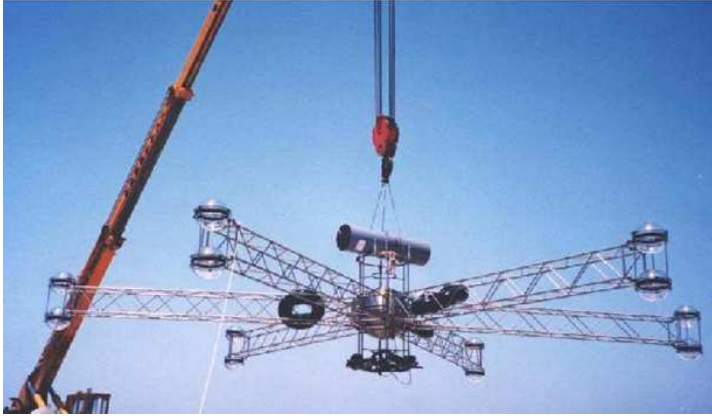
Figure 3. Reduced-size NESTOR floor during preparation for deployment.
