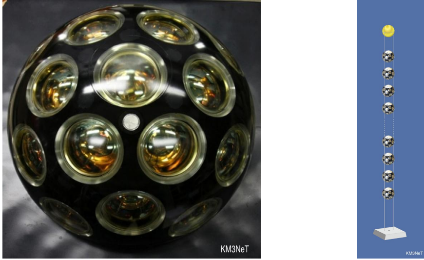
Figure 2.2: Detection modules used in the KM3NeT detector. On the left side a DOM and on the right side a String, which is comprised of multiple DOMs. Taken from [Adr16].
