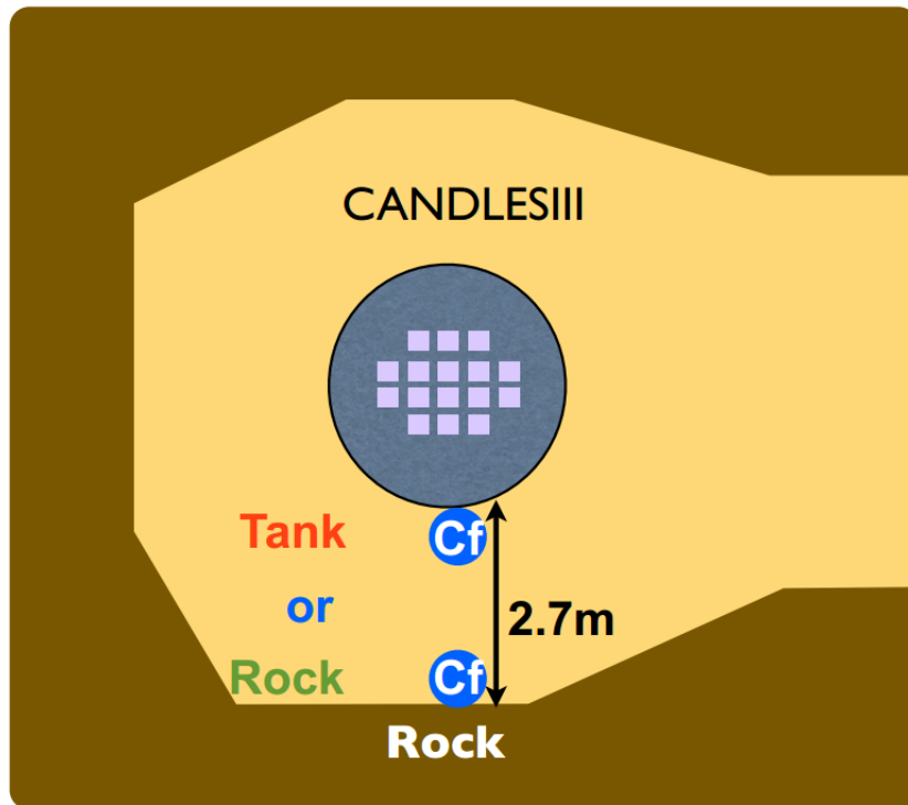
Figure 9.2.: Experimental setup of the ^{252}\text{Cf} source runs for the "Tank" and "Rock" runs. In the first case, the source is attached to the surface of the stainless steel tank and in the latter case it is put close to the southern rock of the cave. [21]
