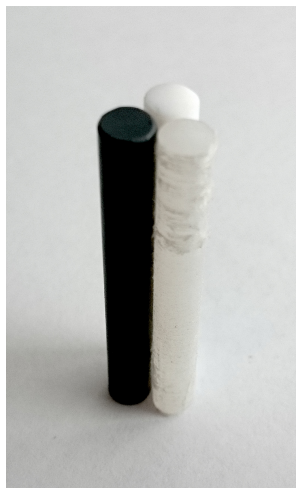
Figure 3.1: Picture of the three plastic rods made of PTFE, PVC, PMMA. The rods are about \varnothing = 5 mm in diameter and about 3 cm in length.
