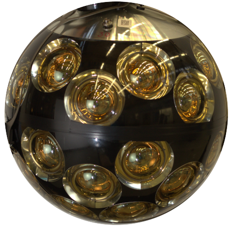
Figure 2.7: Digital optical module (DOM) - Taken from [13].
