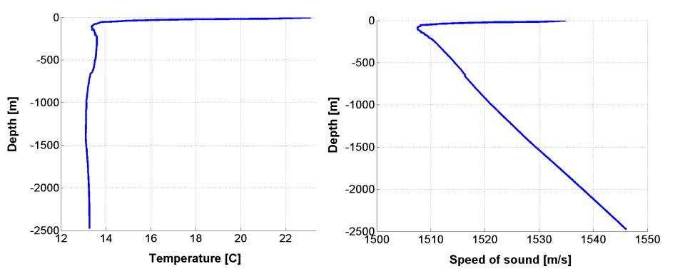
Speed of sound depends on temperature, salinity, pressure (depth); temperature gradient only relevant up to ~100m below surface
