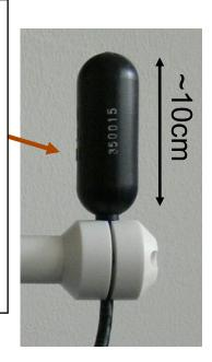
Titanium cylinder with electronics
