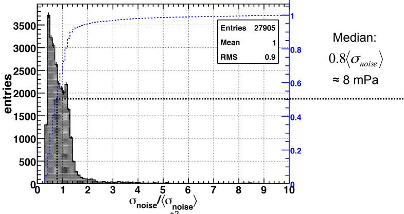
For sensor sensitivity of -145  $^{+2}_{-2}$  dB re 1V/ $\mu$ Pa (lab calibration), the mean noise level is 10 $^{+3}_{-2}$  mPa
