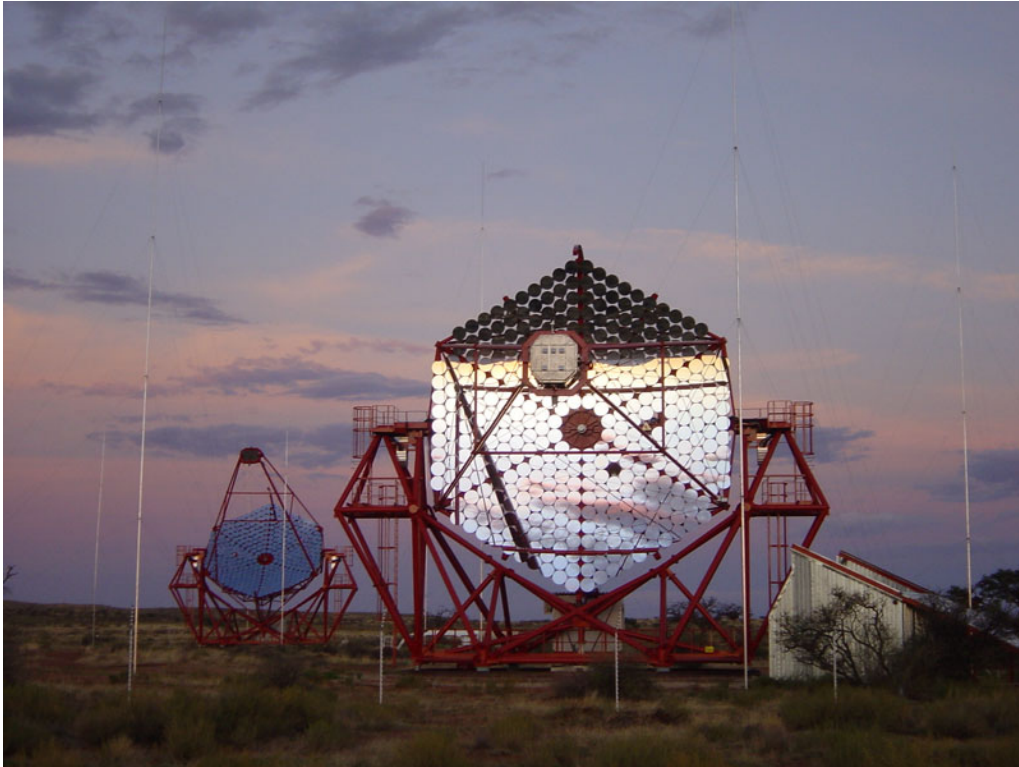
Fig. 3.1: Two of the four 13m H.E.S.S. telescopes, each surrounded by four lightning conductors
