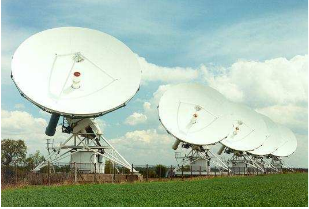
Figure 2.7: The Ryle telescope in Great Britain. The antennas can be moved on rail tracks. The array consists of eight telescopes. Five of them are in a compact configuration here, as the photo was taken. ( www.mrao.cam.ac.uk/telescopes/ryle/ )
