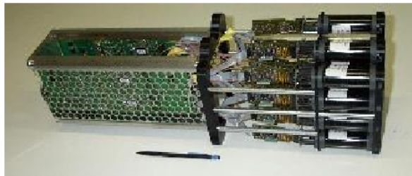
Figure 3.4: Photo of a drawer of a camera. Visible are the 16 PMTs and the corresponding electronics.
