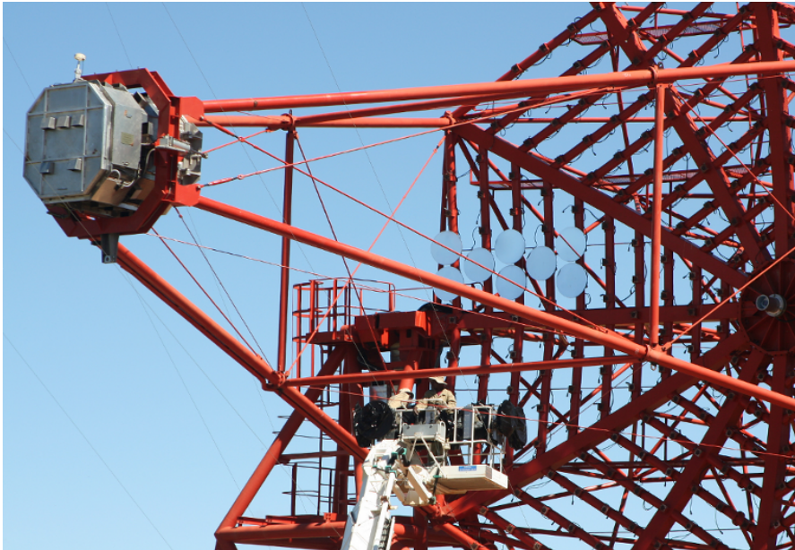
Figure 3.6: The telescope CT3 during mirror exchange in April 2010. The round mirrors each with a diameter of 60 cm are mounted on a steel construction. The camera is positioned on a four arm system in the focal plane with 15 m distance to the reflector plane.
