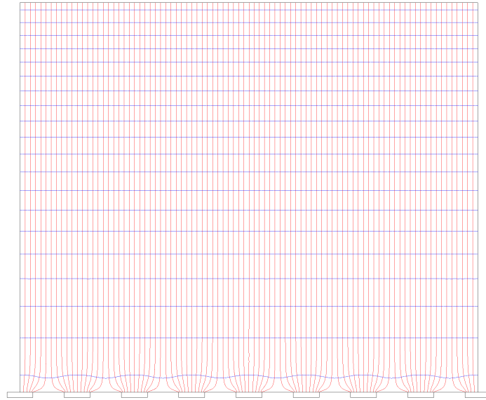
Figure 3.1 Electric field lines (red, vertical) and electric potential (blue, horizontal) for a doped CdTe sensor with the standard setup parameters. The pixelated electrodes are drawn as small boxes at the bottom of the sensor layer. The increase of the electric field strength, i.e. the density of the field lines, close to the pixelated electrodes can be clearly seen. The slope in the electric potential can be observed by the varying distances of the equally separated potential field lines.
