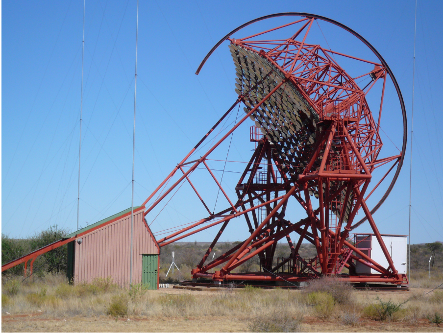
Figure 3.4.: A single telescope of the array, The camera is parked in a shelter to protect the sensitive instruments from the sunlight and rain.
