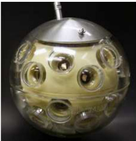
Figure 9: A SeaWiet multi-PMT optical module
