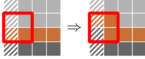
Figure 3.5: Schematic view of the contribution of the first pixel in the next row of pixels to the generating function of the number of equivalent tensor configurations using minus sampling boundary conditions. Hatched pixels lie on the outside of the N \times N pixels region and are used to determine the contribution of boundary pixels. The left hand side shows the state of the pixels before processing the red region, the right hand side afterwards. The color code is the same as in figure 3.1.
