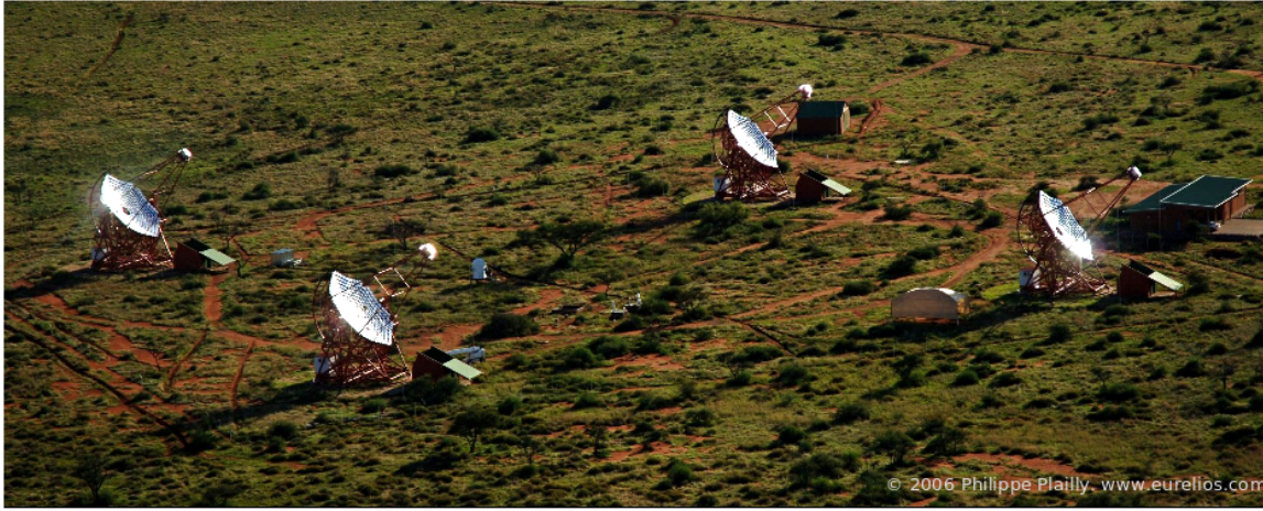
Figure 3.8: The H.E.S.S. Experiment (phase I) with its four IACT telescopes.
