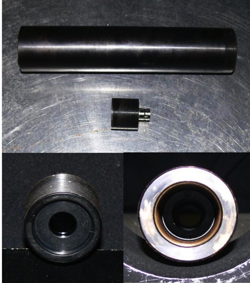
Figure 9.6: Photos of the tube and the PHD. Top: side view of the tube and the PHD, bottom left: front view of the PHD, bottom right: front view of the tube.
