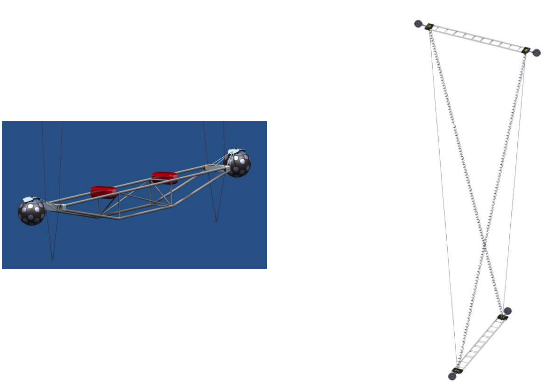
Figure 5.5: The planned storeys in KM3NeT: The left Figure shows the layout of a storey. The Figure on the right illustrates how two consecutive storeys are positioned with respect to each other.
