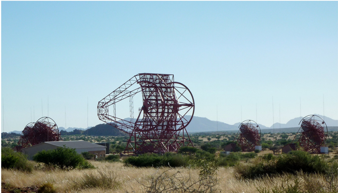
Fig. 3.7: The H. E. S. S. array in Namibia with the four 13 m telescopes and the new central 28 m telescope. The four smaller telescopes are arranged in a square of 120 m length.
