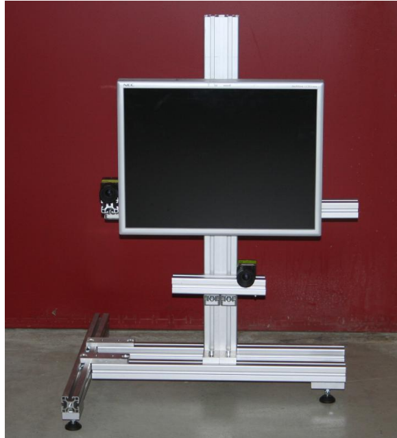
Figure 3.7: LWD-setup used in Erlangen to perform comparing measurements with classical 2f-measurements
