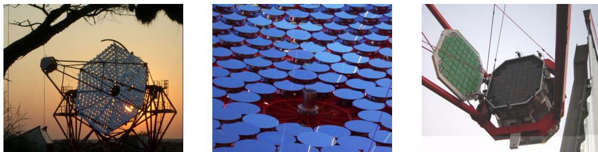
Figure 4.6.: Detailed view of one of the H.E.S.S. 1 telescopes [H.E12]. From left to right the images show the parked out telescope, a close-up view of the mirrors and the camera.
