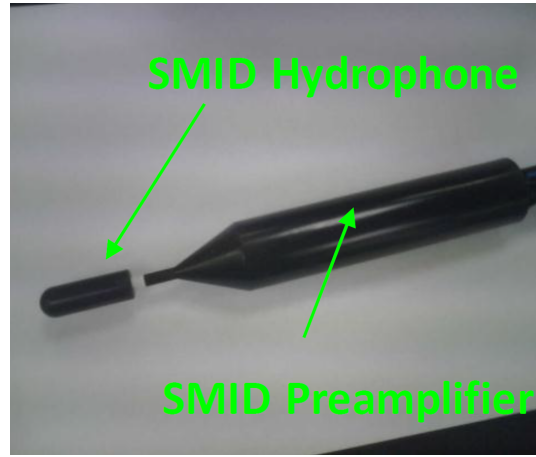
Figure 5.3: A SMID hydrophone with its preamplifier [10]
