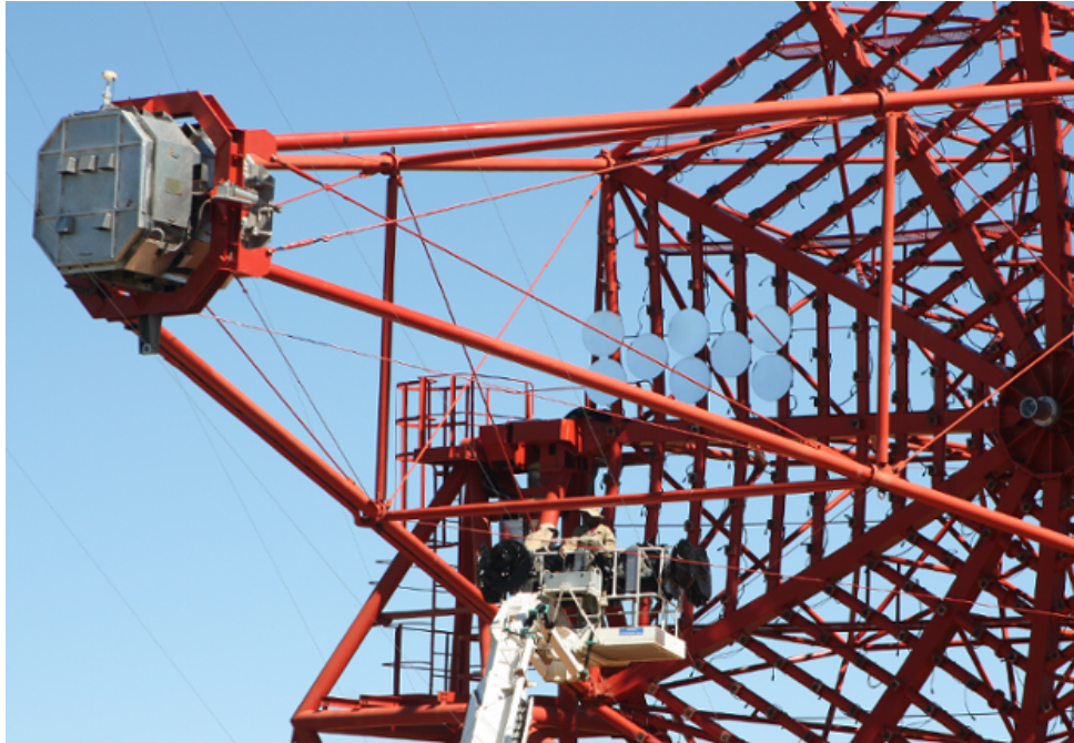
Figure 4.6: The telescope CT3 during mirror exchange in April 2010. The round mirrors, each with a diameter of 60 cm, are mounted on a steel structure. The camera is positioned on a four-arm system in the focal plane with 15 m distance to the reflector plane.
