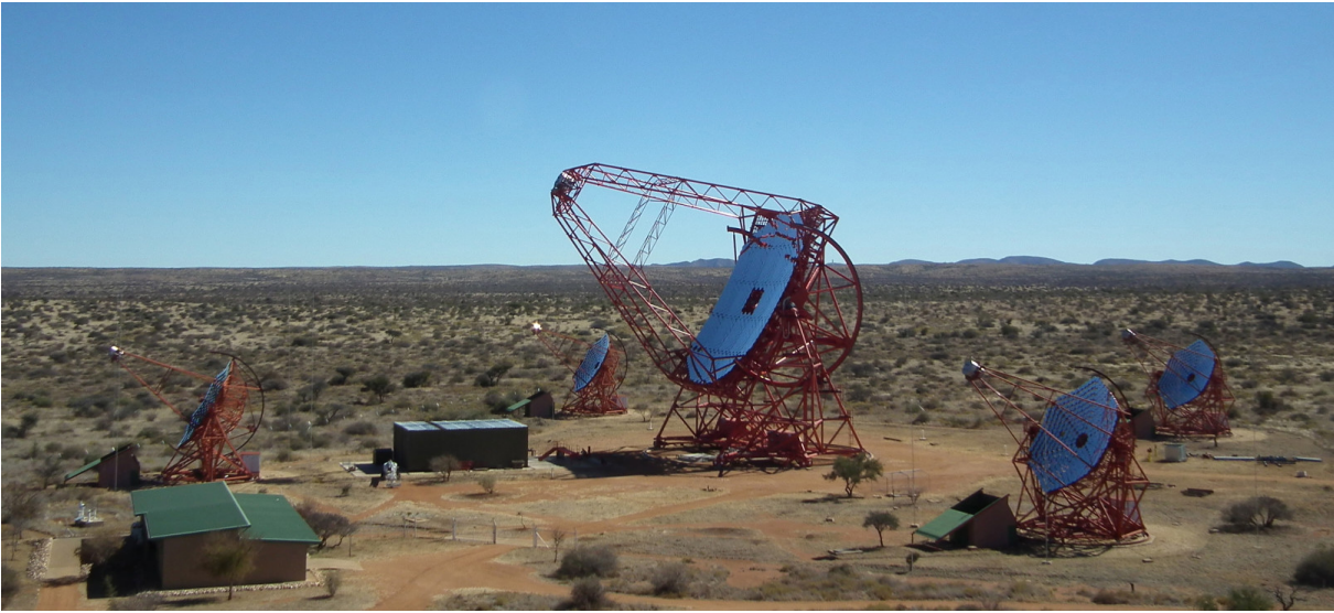
Figure 4.5: View of the full H.E.S.S. array with the four 12 m telescopes and the 28 m H.E.S.S. II telescope (Credit: H.E.S.S. Collaboration, Frikkie van Greunen)
