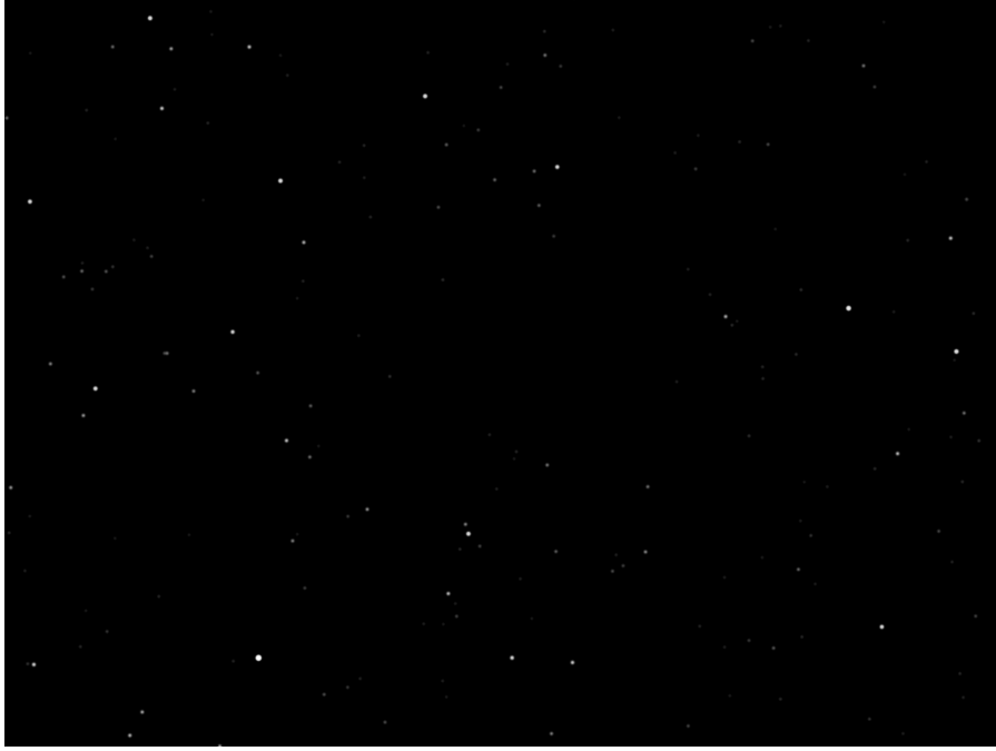
Figure 5.3: A simulated pointing image with the center at (RA, Dec) = (12 h 30 min 49.4 s, +12° 23' 28.0''), the coordinates of M87. The image is simulated with an exposure time of 10 s and an f-number of 1.8.
