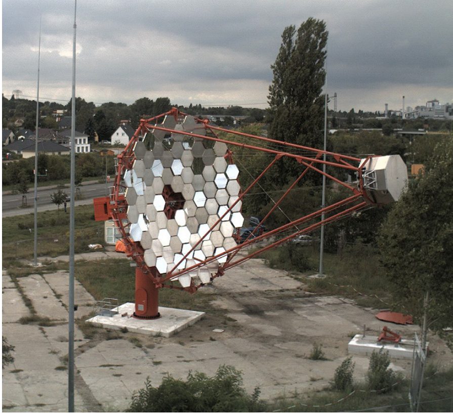
Figure 3.7: The prototype of a medium-sized telescope in Berlin/Adlershof. ( http://www-zeuthen.desy.de/cta\_cam/photogallery1/ )
