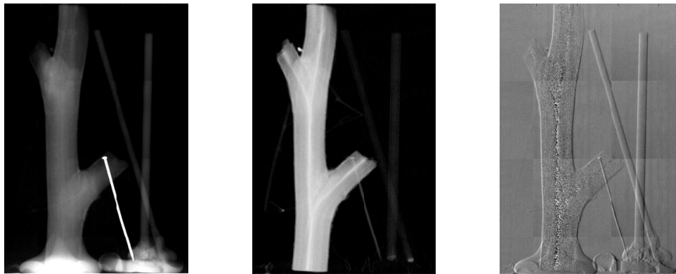
Fig. 1: Attenuation (left), dark-field (middle) and differential phase (right) images of a small branch, a grass stalk, two carbon fibre rods and a metallic needle, fixed with hot glue.
