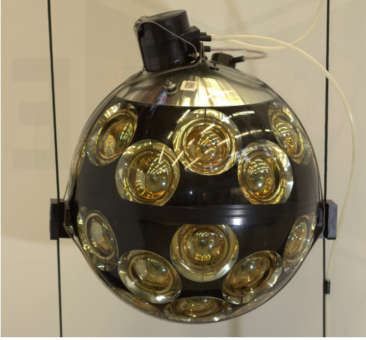
(a) Real KM3NeT-DOM including connector and mechanical mounting. Image taken from [url18a].
