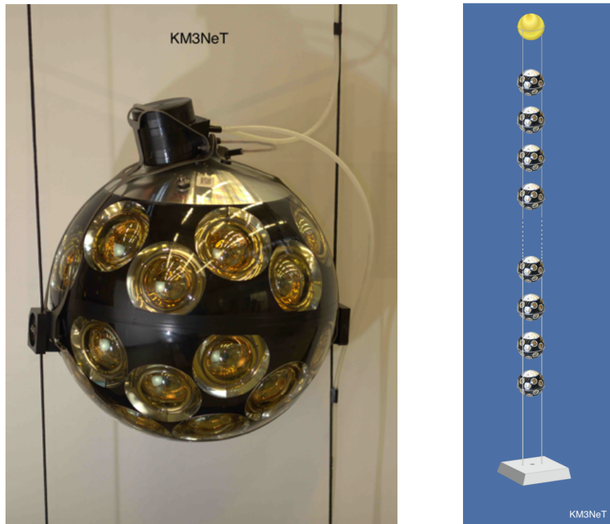
Figure 3.1: Left: The KM3NeT digital optical module (DOM); right: a detection string which hosts 18 DOMs (36m spacing). Figures taken from [AM+16].
