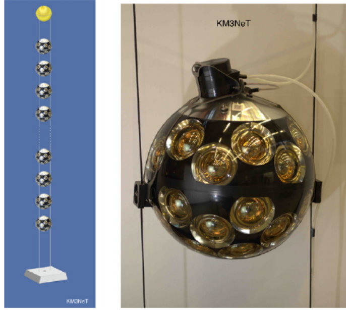
Figure 4.1: String (left) and Digital Optical Module [1]
