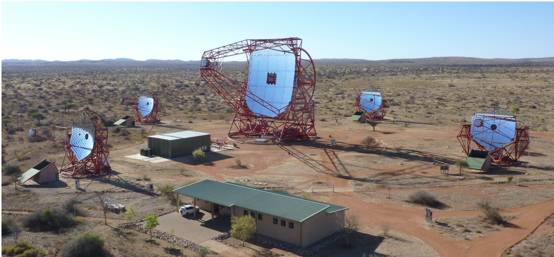
Figure 3.1: The H.E.S.S. \gamma -ray observatory, in its final phase II configuration consisting of five Imaging Atmospheric Cherenkov Telescopes. Image credit: H.E.S.S. Collaboration.
