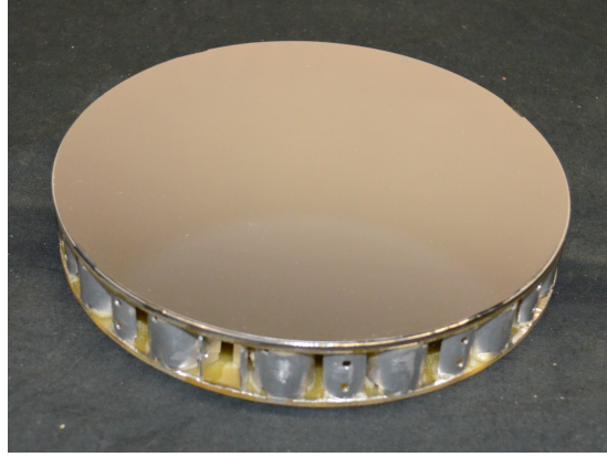
Figure 4.1: Above, a small size mirror at Erlangen Centre for Astroparticle Physics with a curvature radius of 30m and a diameter of 20cm
