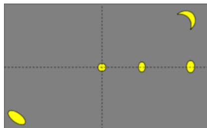
Fig. 3.5 Illustration of the spot deformation. The center spot is the standard appearance of a spot. (Molenaar [16])
