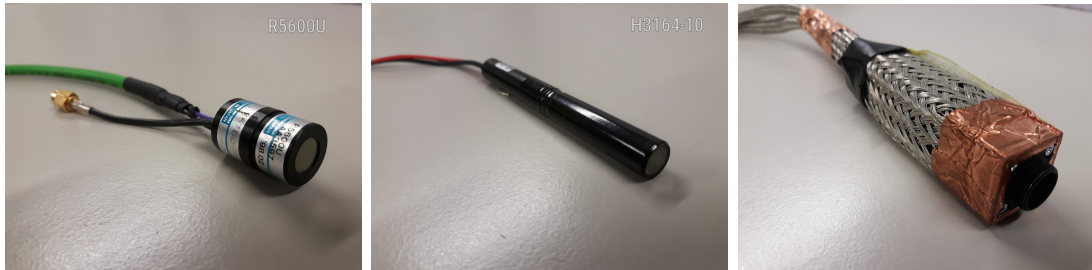
Figure 2.2.: Different photomultipliers used during the measurements: R5600 (left), H3164-10 (center) and H10770-40 (right)
