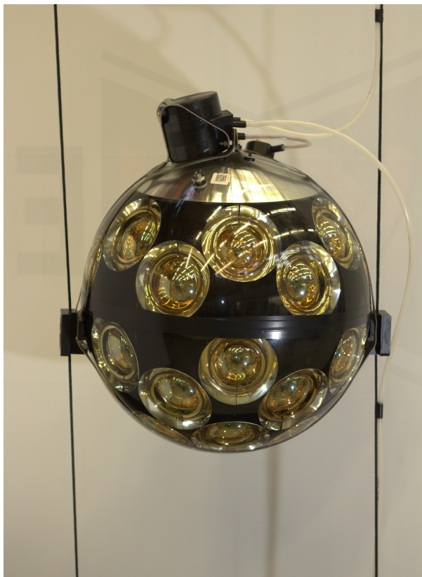
Figure 4: A digital optical module (DOM) used for KM3NeT. (credits: KM3NeT)
