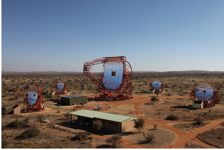
Figure 2.4. – H.E.S.S. with all five telescopes. CT1-4 are arranged in a square of 120 m side length [38]. CT5 is located in the middle of the square. Figure from Ref. [2].
