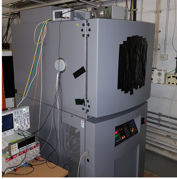
Figure 11: Temperature-Chamber used for module calibration.
