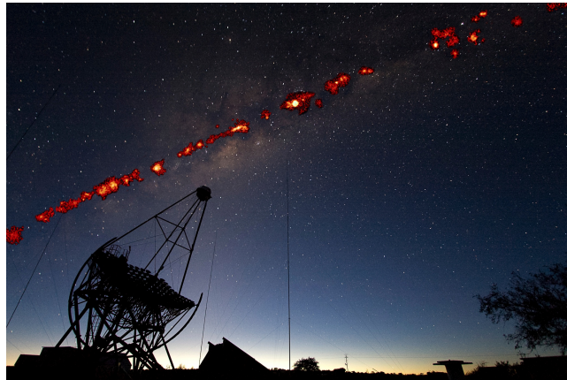
Figure 1.1: Photo montage of the night sky over Namibia with the H.E.S.S. map of the galactic plane survey. The telescope in the foreground is one of the small H.E.S.S. telescopes. The red spots in the background are VHE gamma-ray sources observed by H.E.S.S. [4].
