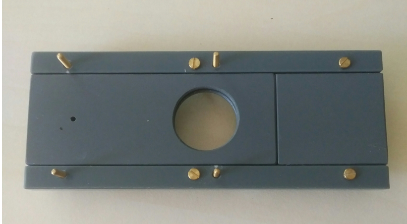
Figure 3.3: Containment for the sources used in the setup
