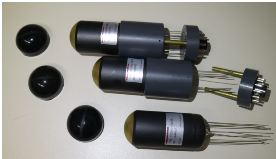
Figure 4.5: PMTs with encasements (consisting of two separable parts), which were developed in collaboration with the ECAP mechanics workshop. The encasements contain HAMAMATSU sockets with gold contacts to contact the flying leads of the PMTs and can be easily plugged in the voltage divider cluster.
