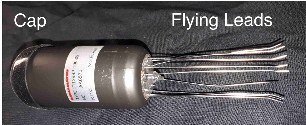
Figure 2.2: Sample PMT of the 7 dynodes type. Cathode, dynodes, and anode are contacted by flying leads, which ease the soldering process into the FlashCam modules later on. A removable rubber cap over the entrance window protects the PMT from light during the transport.
