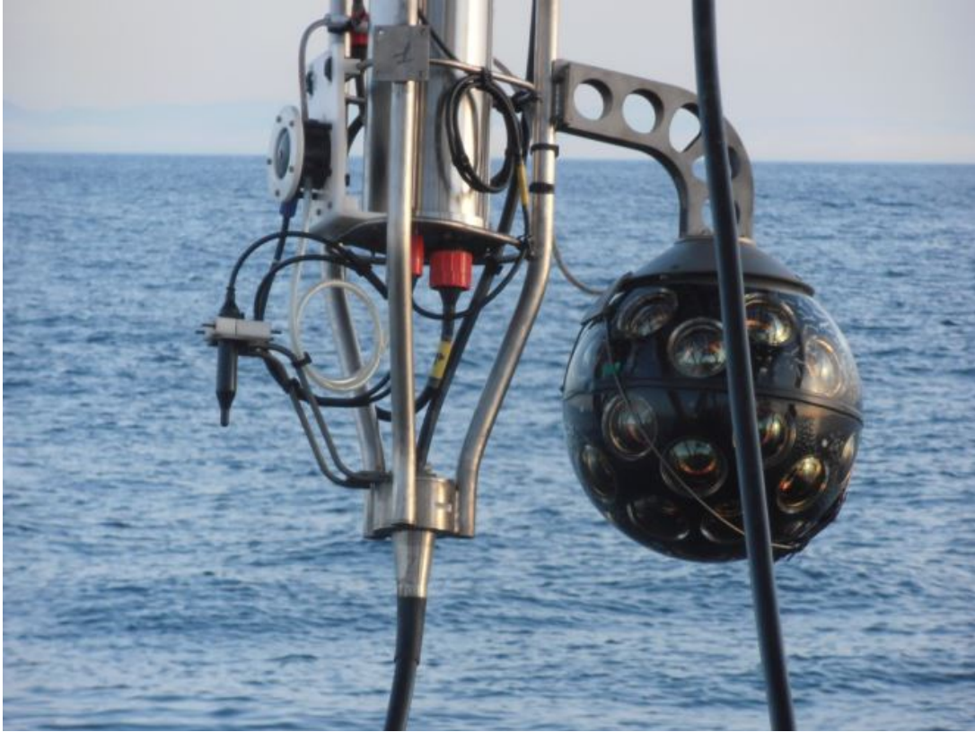
Figure 10.1: Photograph of the KM3NeT PPM-DOM mounted at the ANTARES instrumentation line. Figure taken from [37].
