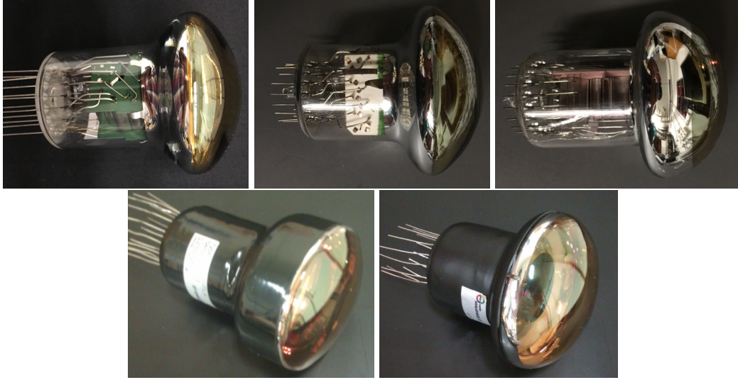
Figure 6.1: Photographs of PMT candidates for KM3NeT. From top left to bottom right: Hamamatsu R12199-02, HZC XP82B20, MELZ FEU, ETL D783KFLA, ETL D792KFLA.
