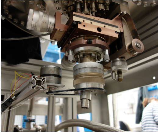
Figure 3.17.: 4-axial feedthrough for the PMT suspension on the bottom of the main chamber. The stepping motor can be seen on the left.
