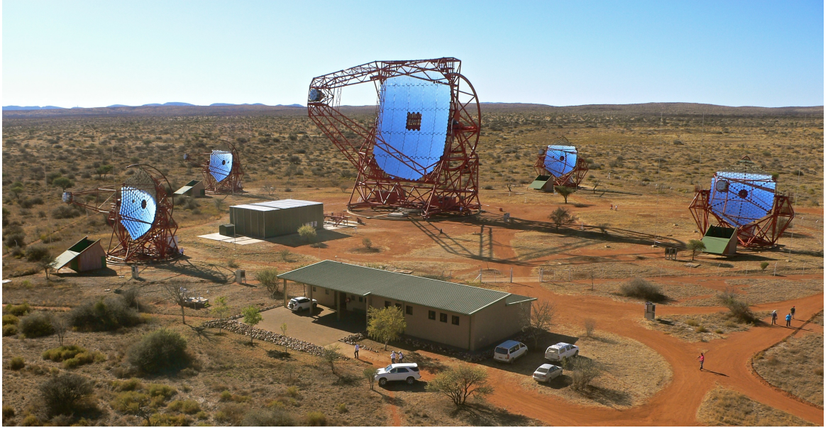
Figure 2.2: Photograph of the complete H.E.S.S. telescope array with the four smaller telescopes CT1-4 and its large telescope CT5 in the centre. Image credit: H.E.S.S. Collaboration.
