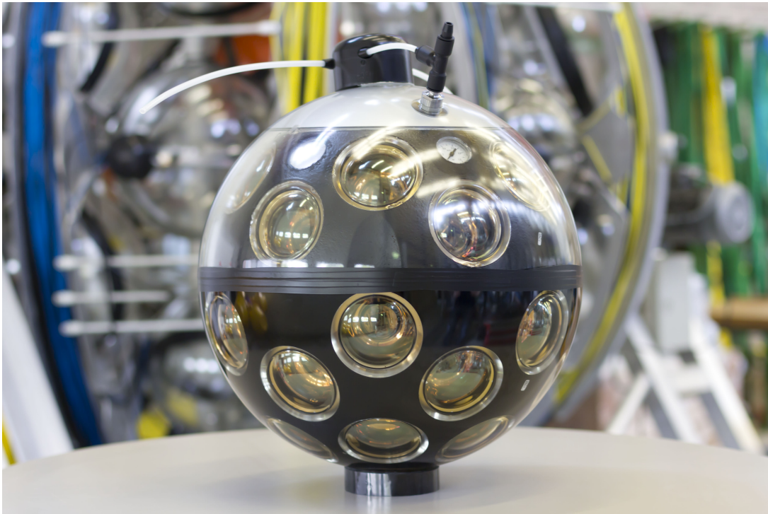
Figure 3.2: The KM3NeT DOM with 12 PMTs in two rows on the upper hemisphere 18 PMTs in three rows on the lower hemisphere and one PMT pointing directly downwards. Picture taken from [7].
