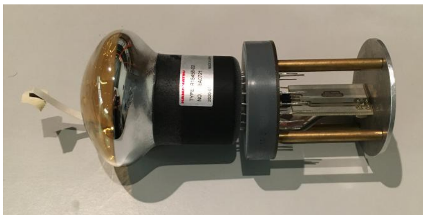
Figure 2.2: PMT (left side) with passive base (right side).
