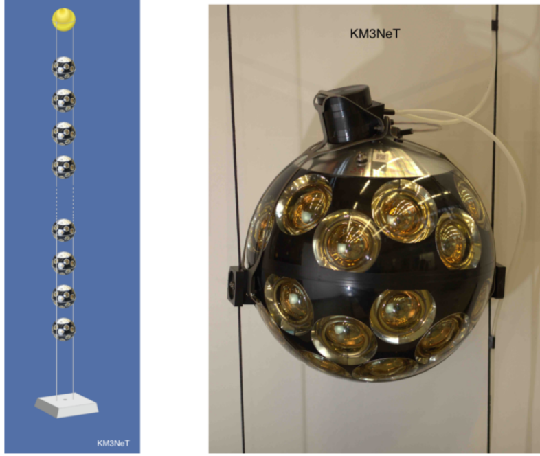
Figure 2.7: Detection string (left) and digital optical module (DOM) for KM3NeT [5].
