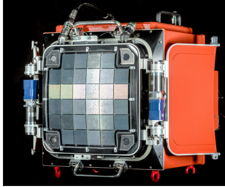
Figure 12: The prototype camera CHEC-S used for SST (picture taken from [17])
