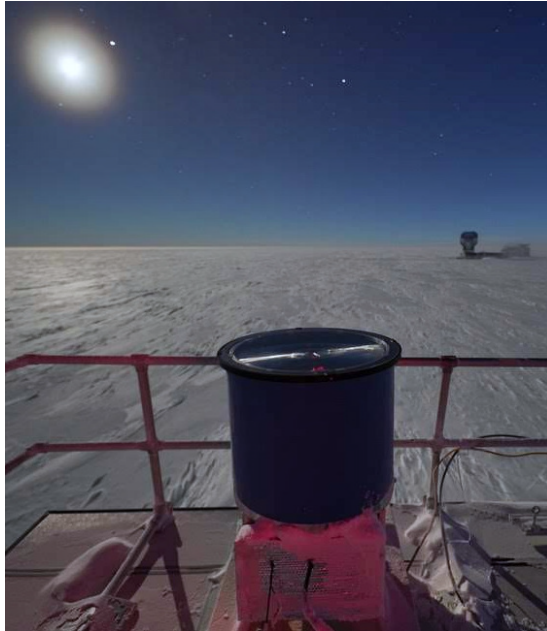
Figure 4.1: Picture of a IceAct prototype telescope in operation[23]
