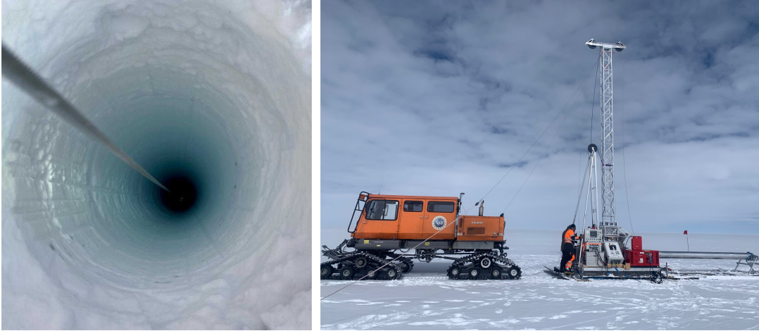
Figure 4.7: Left: Helper string hole of station Amaroq made with the BigRAID drill, the first completed station-hole of RNO-G. Right: BigRAID drill with erected tower and lowered drill. The drill is attached to TUCKER (owned by Summit Camp) to move the drill to the next station after hole completion.
