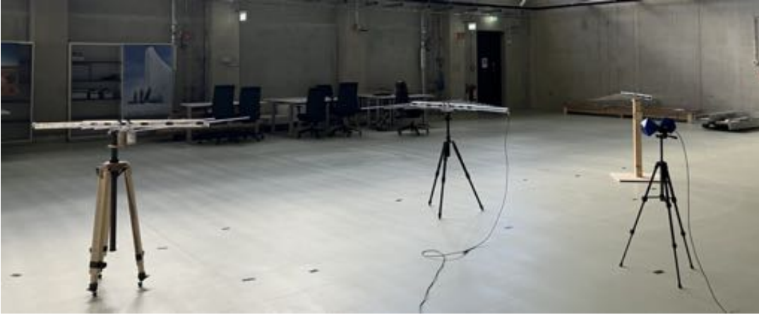
Figure 6.13: Photo of the measurement setup for the RNO-G three antenna setup in free space for 3 m spacing between LPDAs. The blue antenna on the right is the radiating antenna and the middle LPDA (center of the picture) is the receiving antenna.
