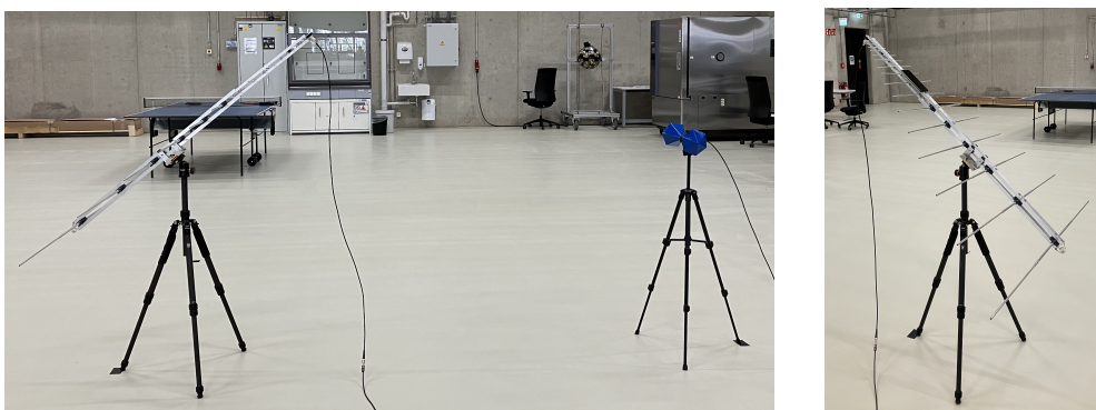
Figure 6.11: Photographs of the setup for vertical radiation pattern measurement for 45^\circ on the left. The blue antenna on the right is the radiating antenna and LPDA on the left is the receiving antenna. On the right is the position of the phone with the phyphox app for adjusting the antenna to the right inclination.
