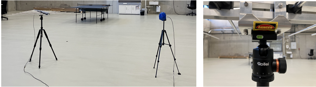
Figure 6.9: Photographs of the setup for horizontal radiation pattern measurement for 105^\circ on the left. The blue biconical antenna is the radiating antenna and the LPDA on the left is the receiving antenna. On the right the rotational angle scale is shown, which is used to identify the angle.
