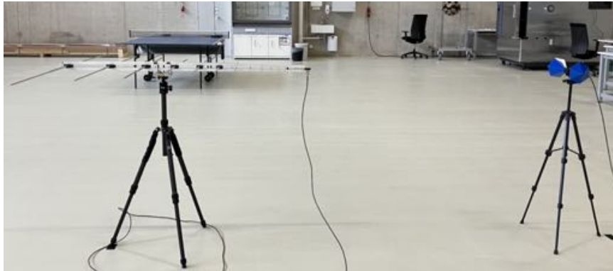
Figure 6.1: Picture of the setup for the distance variation in the experimental hall. biconical as the emitter (on the right) and LPDA as receiver (on the left) face each other directly.
