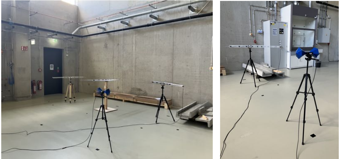
Figure 6.15: Picture of the setup with three LPDAs next to the wall on the left. The blue antenna in the middle of the picture is the radiating antenna and the rightmost antenna is the receiving antenna. On the right the setup with one LPDA is shown.
