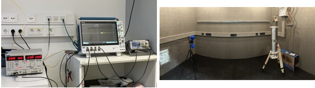
Figure 5.1: Photograph of the radio chamber setup. On the left: instruments outside the chamber (from left to right: voltage source for amplifier, amplifier behind oscilloscope and function generator). On the right: inside of the chamber with the biconical antenna on the left and the Vpol on the right.
