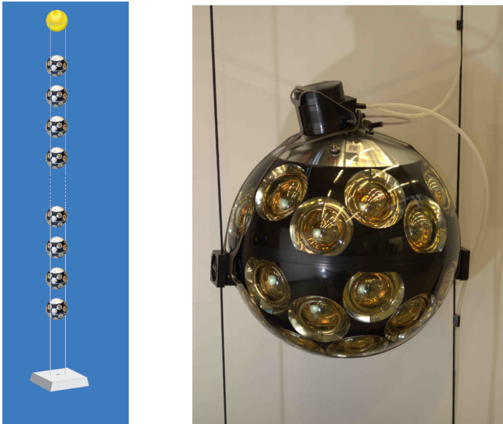
Figure 2.11: Sketch of a KM3NeT detection string ( left ) and a picture of a DOM ( right ) (Adrián-Martínez et al., 2016)
