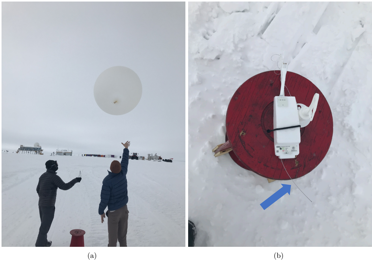
Fig. 3: Picture of (a) a balloon launched at Summit Station (ICECAPS project) and (b) corresponding radiosonde. The blue arrow points at the antenna of the radiosonde. [22]
