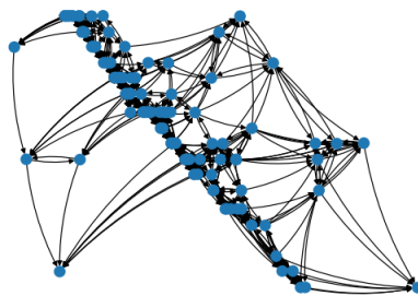
Figure 5.3 – Graph representation of a random event, where each node represents a hit, and each node is connected to its eight nearest neighbors by edges in terms of the euclidean distance in x , y , z and t . The arrows are pointing away from the neighbors, and towards the central node[24].
